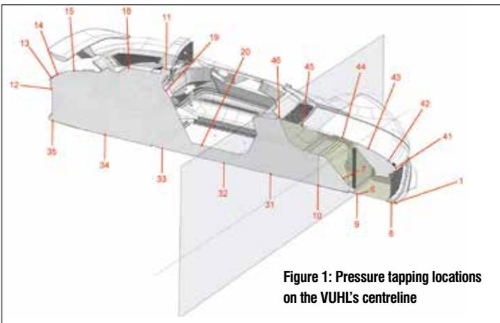
Figure 1: Pressure tapping locations on the VUHL's centreline
