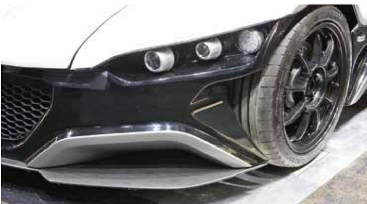
Picture 3: Front splitter and cutaway airdam in front of the front wheels
